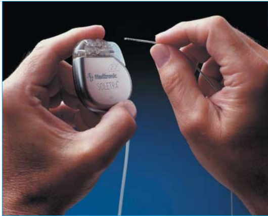
The pacemaker's electrical signals are delivered to the brain through a thin, implanted wire with electrodes attached at the tip.
